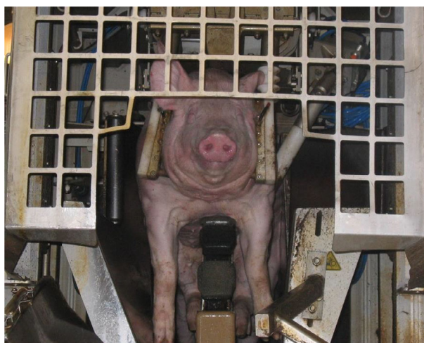
Figure 12: Head-to-body electrical, stunning/killing (three points) and restraining system (source: Virginie Michel)
